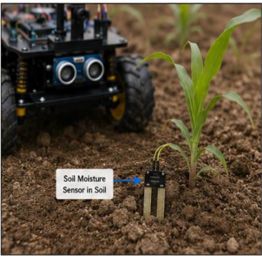
Fig. 6.4:Soil Moisture Sensor-Based Field Monitoring
